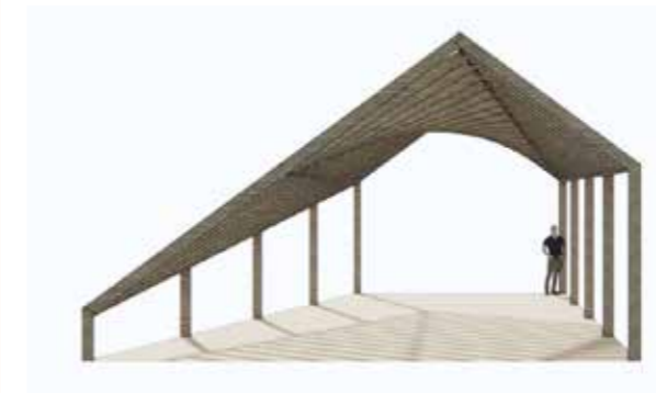
Timber Frame Rear View
